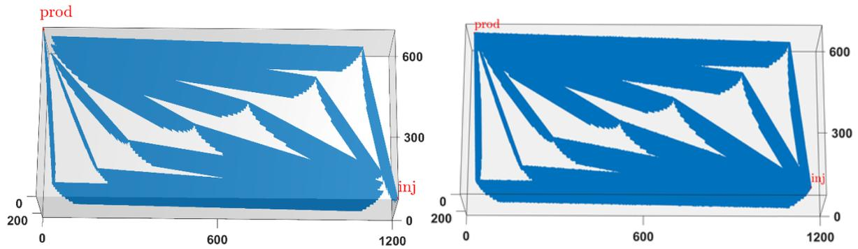
Figure S-3— Simulation domains for the coupled thermal and hydraulic simulation of (a) doublet of fourteen SDF-series, and (b) doublet of fourteen SDF-parallel
