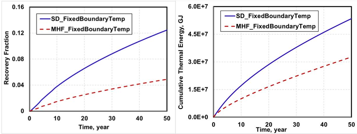
**Figure S7.** Thermal recovery fraction and cumulative thermal energy plots for the expanded grid cases that have no-flow and constant-temperature boundary conditions.
