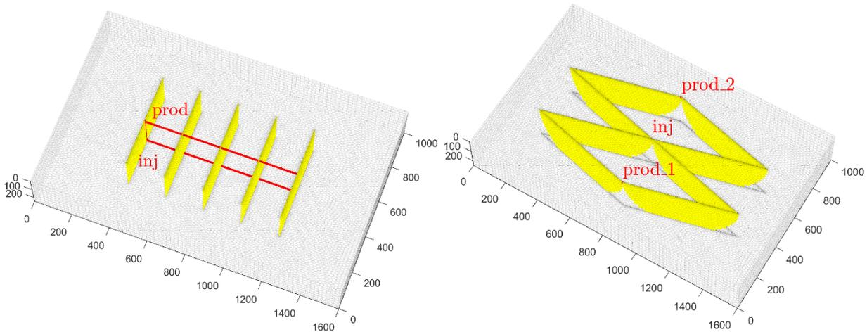
**Figure S5.** Extended grid for the MFHW case and the SDF triplet case with and without constant temperature boundary conditions
