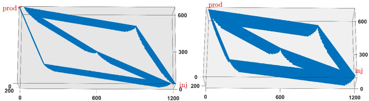
Figure S-1— Simulation domains for the coupled thermal and hydraulic simulation of (a) doublet of six SDF-series, and (b) doublet of six SDF-parallel
