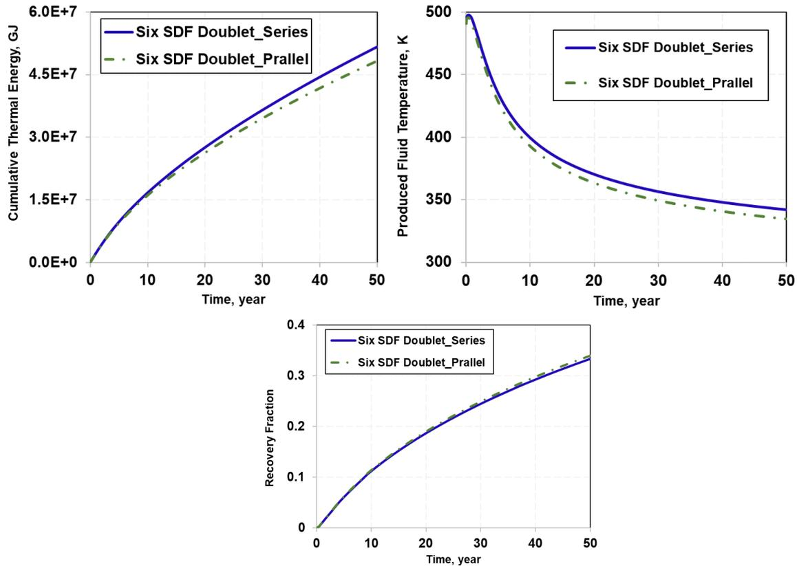
Figure S-2— Comparison of performance between two configurations of the SDF doublet case. (a) comparison of the produced fluid temperature. (b) comparison of cumulative thermal energy (c) comparison of recovery fraction
