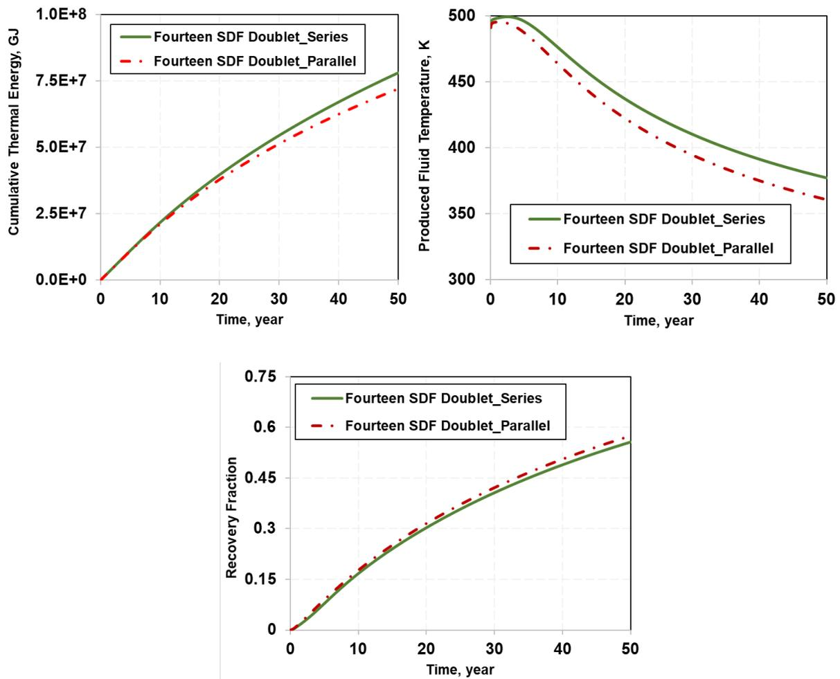
Figure S-4— This figure presents line plots that compare the performance of the series and parallel configurations of the 14 SDF doublet case. It presents a (a) comparison of the produced fluid temperature, (b) cumulative thermal energy, and (c) thermal recovery fraction.
