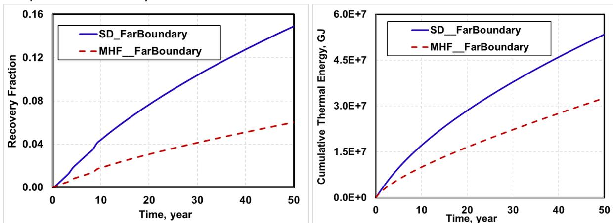
**Figure S6.** Thermal recovery fraction and cumulative thermal energy plots for the expanded grid cases that have no-flow and insulated boundary conditions.
