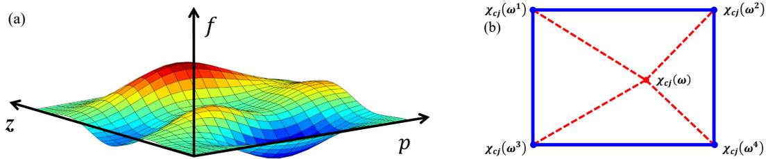
**Fig. 7.** Schematic description of operator parameterization and interpolation process for  $\chi$  operators with a predefined OBL resolution (modified from Voskov (2017); Lyu et al. (2021a)).  $\omega^1$  to  $\omega^4$  are four supporting points, and  $\omega$  is the current thermodynamic state of a given control volume at a given timestep in the simulation. (a) Operator distribution and (b) interpolation.
