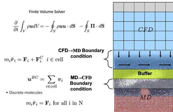
**Fig. 4.** A domain decomposition coupling arrangement, which includes: (1) an averaged region at the bottom boundary to determine the CFD boundary, and (2) a constrained region at the top boundary of the domain where a termination force is applied to prevent molecules from escaping. Additionally, a buffer zone is incorporated to ensure that the constrained molecular region does not directly interact with the averaged region used for boundary determination (Smith and Theodorakis, 2024).
