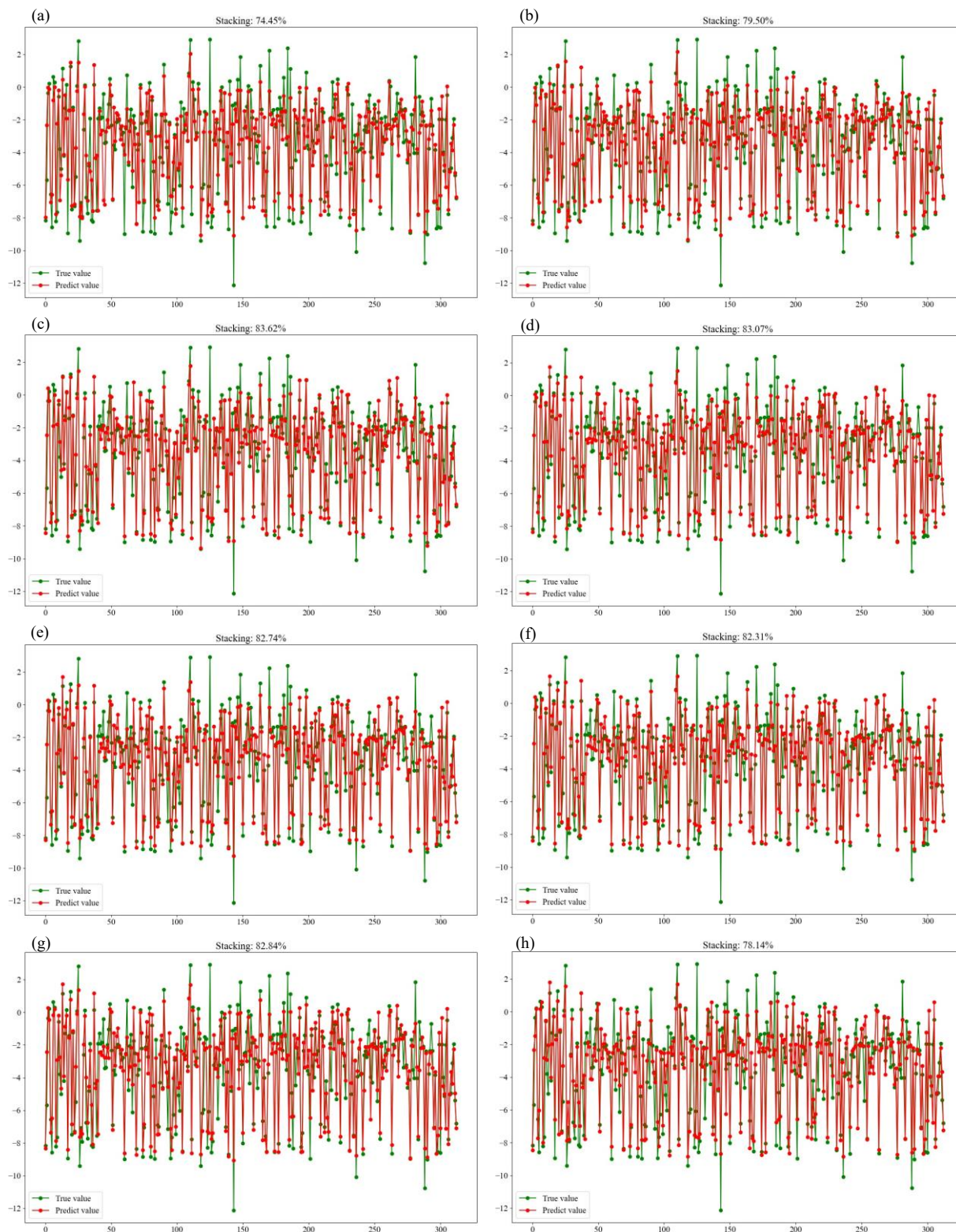
Fig. S5. The R^2 results of feature ablation study for Stacking permeability prediction models. (A)Depth; (B)Depth, DEN; (C) Depth, DEN, SP; (D) Depth, DEN, SP, GR; (E) Depth, DEN, SP, GR, CNL; (F) Depth, DEN, SP, GR, CNL, CAL; (G) Depth, DEN, SP, GR, CNL, CAL, AC; (H) DEN, SP, GR, CNL, CAL, AC.
